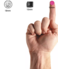
10 by 10 mm is a good minimum touch target size. (Image source: UXmag)
